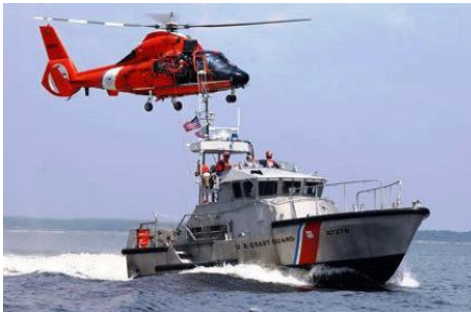
Figure 3.2 - CG HH-65 Helicopter Conducting Hoisting Operations with a CG 47-foot Small Boat
