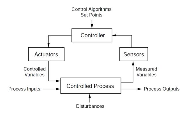
Figure 1 A standard control diagram (Leveson, 2011, pp. 66)
