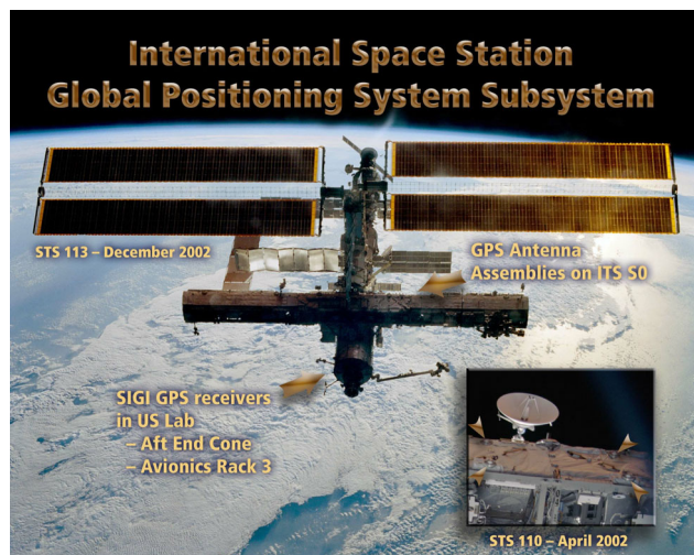
Figure 1B – ISS GPS Subsystem
